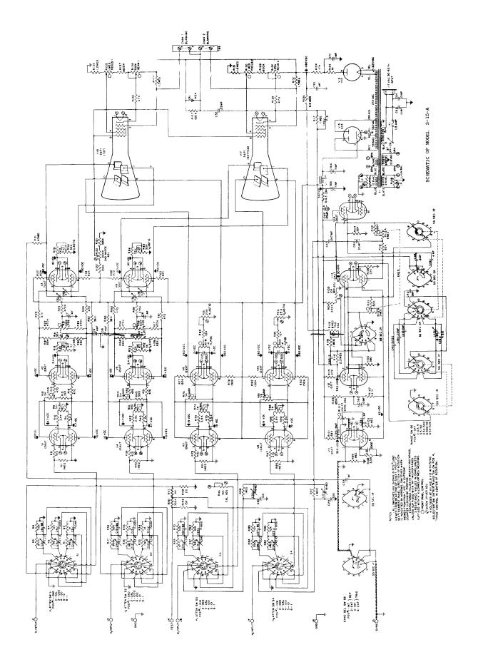
The linear time base generator is common to both cathode ray tubes when their respective H ATT switches are set to SW. The generator is a multivibrator type which produces a linear sawtooth voltage in either the repetitive or trigger mode of operation.
